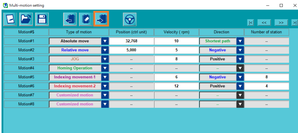
Figure 5.1.1 Save the parameters to servo drive
